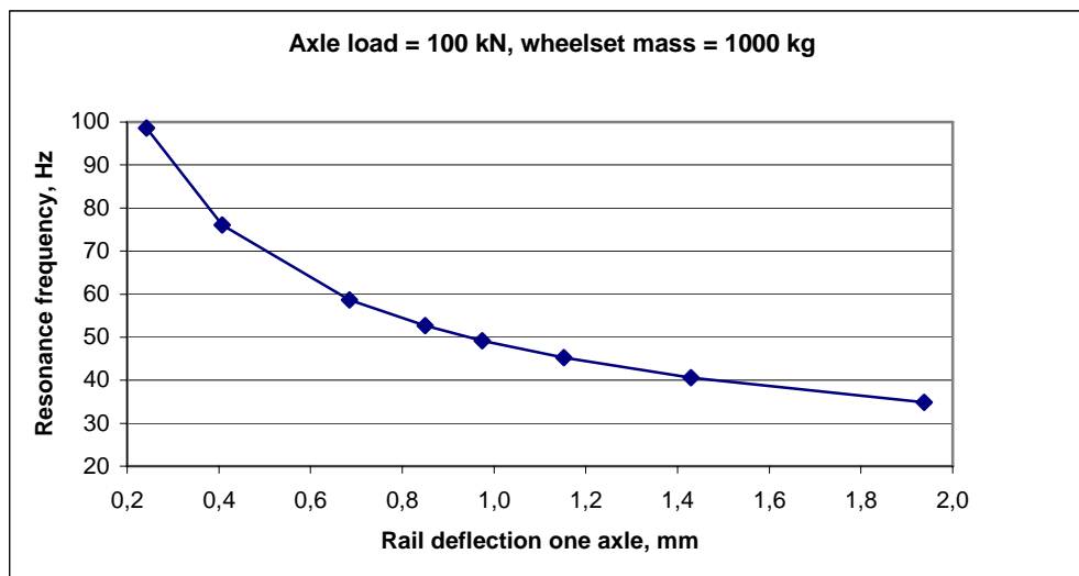
Fig 9. Resonance frequency as a function of rail deflection. Axle load = 100 kN. Ri60N rail. Mass of wheel set = 1000 kg. Relation k_{\text{acou}} / k_{\text{dyn}} = 1.2 .
