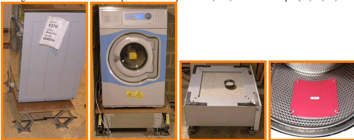
Figure 1. Washing machine Electrolux Laundry Systems type Wascator 465H*, on a) the framed base with a MDF plate on 4 hand-operated jacks, b) the concrete filled steel plate base (200 kg) resting on
